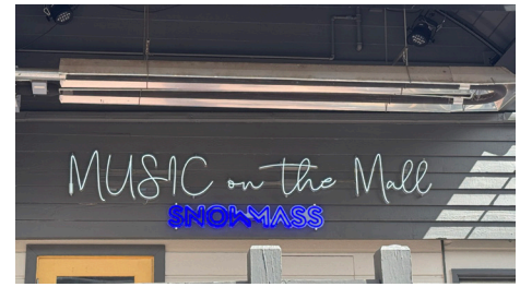
Figure 19. An example of a “neon-look” LED.
