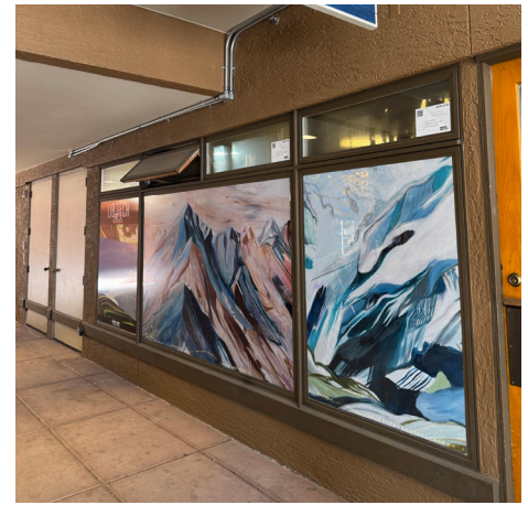
Figure 11. Window clings may be used in service areas where privacy is desired or used to mask ‘back of house’ areas.
